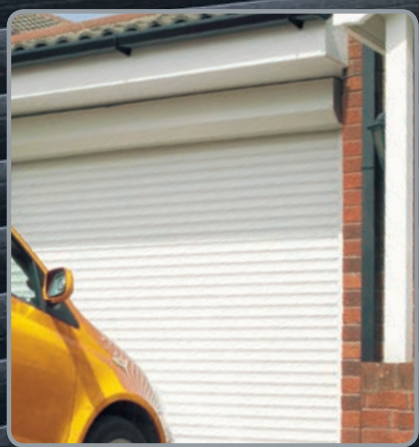
Doors can be fitted externally if headroom is very limited inside the garage. The roll box will be visible and the concave face of the door slats faces outwards.
